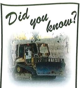
A dozer's fire line plays a crucial role in extinguishing wildland fires. These lines, created by using the front 10-foot blade, are placed ahead of a fire, flammable removing plant material down to bare soil. leaving nothing for the fire to burn. Fire containment expressed as a percentage of a wildfire's perimeter that surrounded by a control line. For instance, if a wildfire is 25 percent contained, control lines 25 percent around of perimeter have been established.
