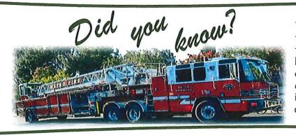
Tillers are the District's longest trucks and are equipped with ladders that can extend over 100 feet. They have a cab at the rear, which is driven by a firefighter. Although it can be 60 feet long, it can maneuver in tight locations, like a narrow road or an apartment parking lot.
